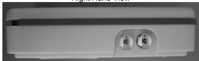
Right hand view showing two gas inlets. The far inlet is for the gas sample for analysis. The near inlet is for the pressure measurement.
